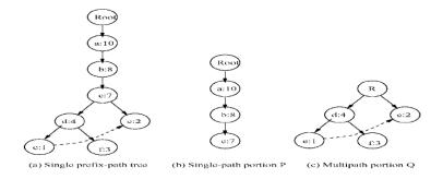
Figure 2.2: Mining an FP-tree with a single prefix path (taken from [22]). The dotted lines are the vertex links.
