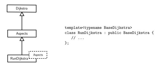
Figure 2.3: UML class diagram providing the idea of our class hierarchy. Aspects are given to RunDijkstra as a template argument.
