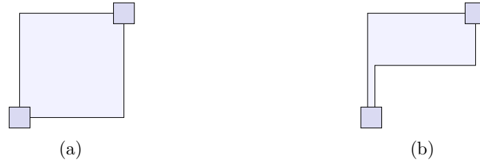
Figure 3.1: There is only one orthogonal representation for \mathfrak{G}_1 where every edge has at most one bend, as seen in Figure (a). In Figure (b), there is a 0^\circ -angle at the lower vertex, at the cost of having two bends in an edge.
